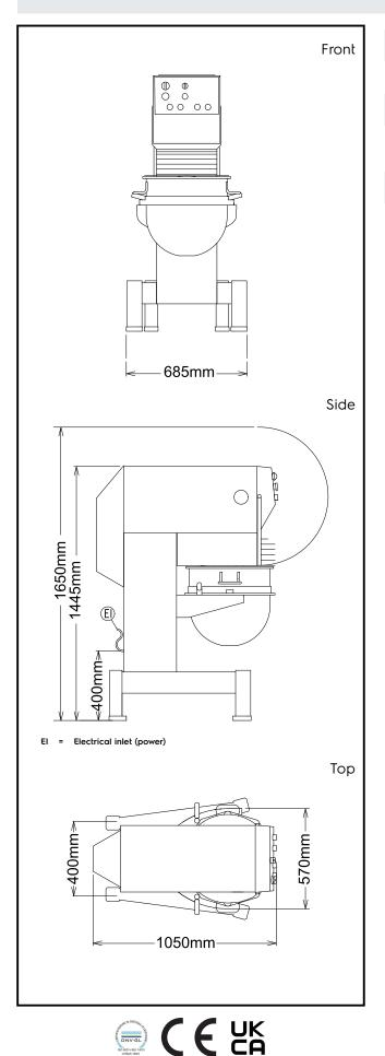
Electric Supply voltage: 380-440 V/3N ph/50/60 Hz 600284 (XBE60X3B) Capacity: ISO 9001; ISO 14001 kg/ Performance (up to): Cycle Capacity: 60 litres
